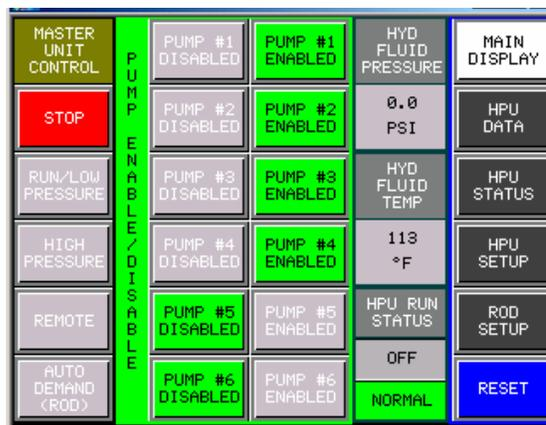
2. If not already displayed, press the **Main Display** button to open the **Main Display** screen.
