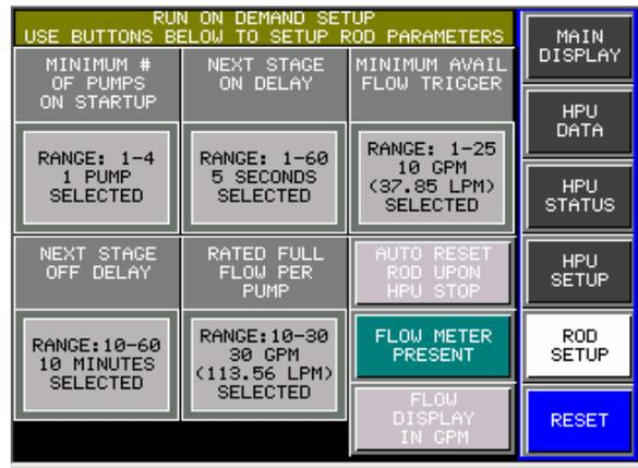
**Flow Meter Present** must be selected to display the contents of this screen.
