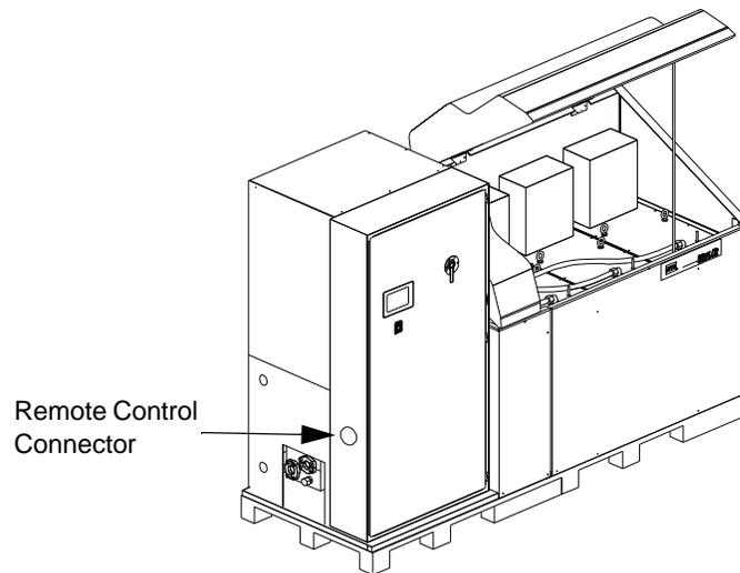
**Note** *If a controller is not used, the installed jumper plug must be used or the unit will not start.*
