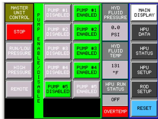
Click on the **HPU Status** button to display the **HPU Status** screen and identify the fault conditions (see the next figure).
