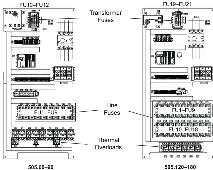
Reset the thermal overload switches or replace the fuses as follows:
