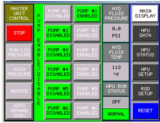
2. Press the **Pump #\_ Enabled** for the first pump to be adjusted.
