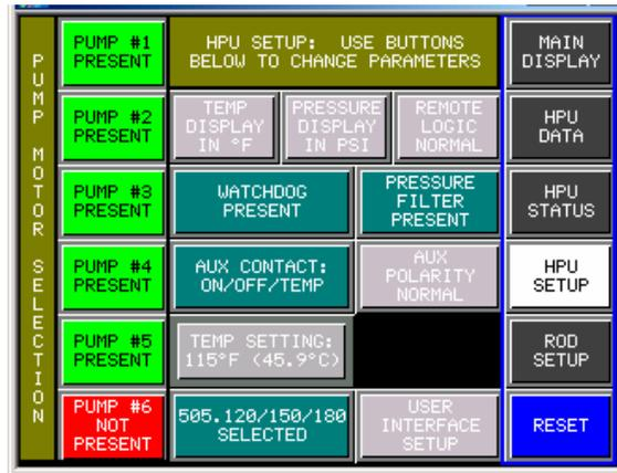
6. Verify that the correct pumps are present for the HPU model installed.
