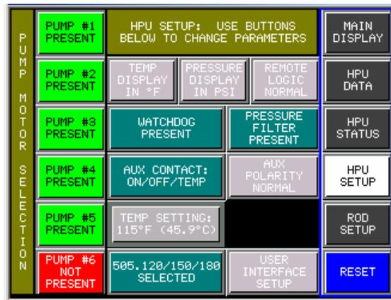
To select this screen you must press and hold the **HPU Setup** button for five seconds.
