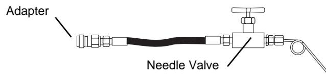
**Hose Valve Assembly for Fluid Sampling**
