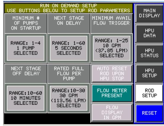
From the current screen, press and hold the **ROD Setup** button on the user interface for five seconds. When the **ROD Setup** screen displays, if only the **Flow Meter Not Present** button is displayed, press this button to display the setup parameters buttons.
