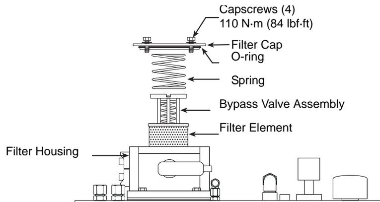
The return-line filter element of the HPU should be replaced for the following reasons:
